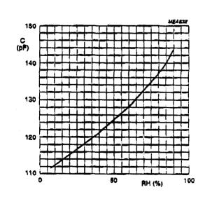
Fig.2 Typical capacitance as a function of relative humidity.
